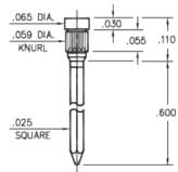
**Description:** 1094 - Wire Wrap Terminal Pin **Packaging:** Packaged in Bulk
