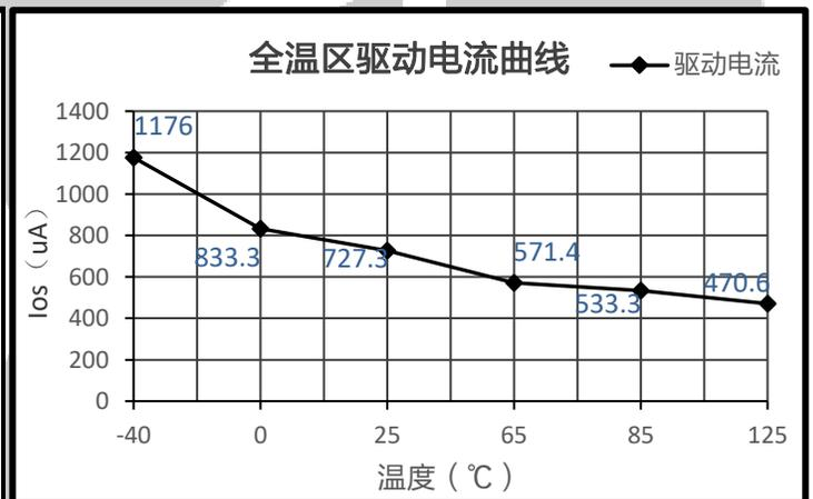
Figure 3.  $I_{OS}$  Curve In  $-40^\circ\text{C} \sim 125^\circ\text{C}$
