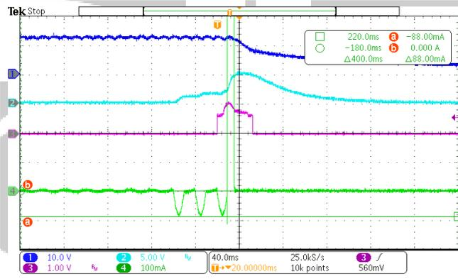
CH1: VS(PIN8),10V/div CH2: OA(Pin7),5V/div
