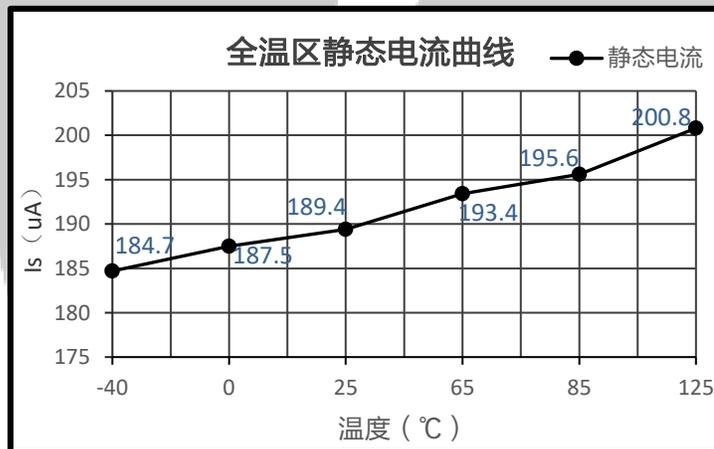
Figure 2.  $I_S$  Curve In  $-40^\circ\text{C} \sim 125^\circ\text{C}$
