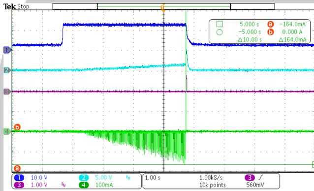
CH1: VS(PIN8),10V/div CH2: OA(Pin7),5V/div
