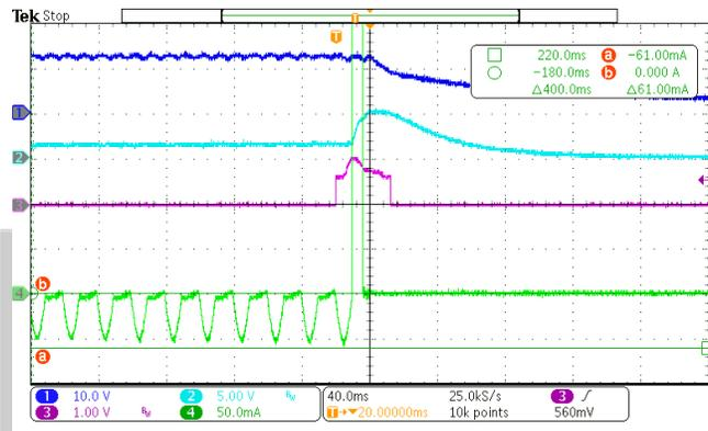
CH1: VS(PIN8),10V/div CH2: OA(Pin7),5V/div
