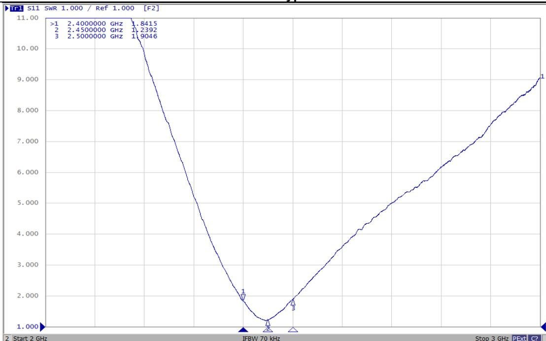
**Antenna on Type-2 Test Board**
