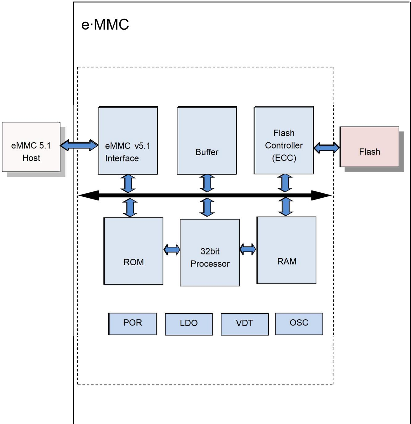
Figure 1 - e-MMC Block Diagram
