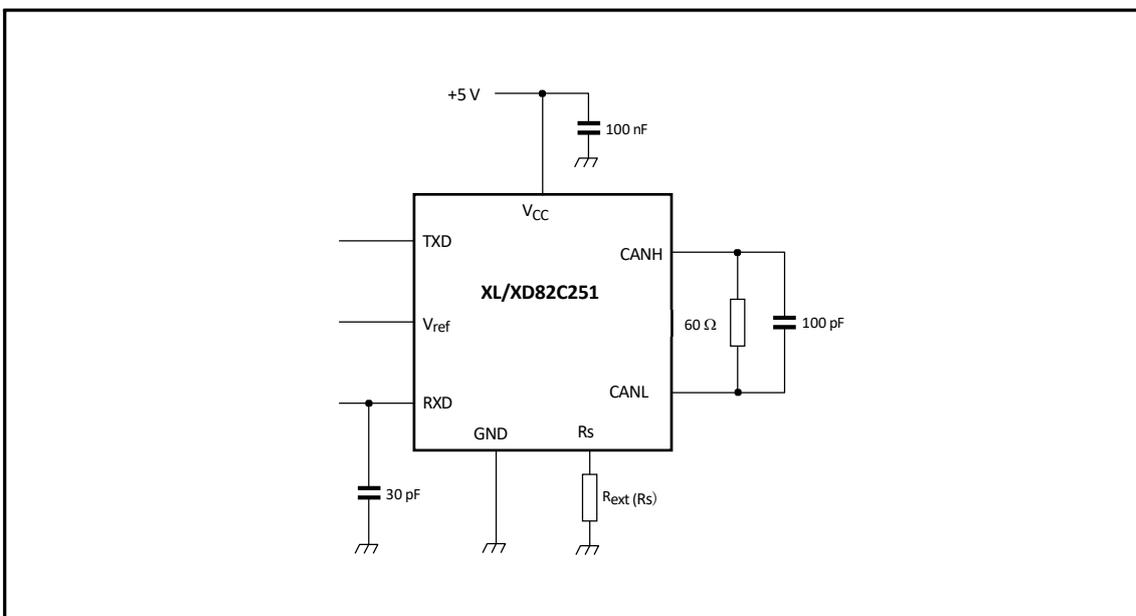
**Figure 6-1 : Test circuit for dynamic characteristics**
