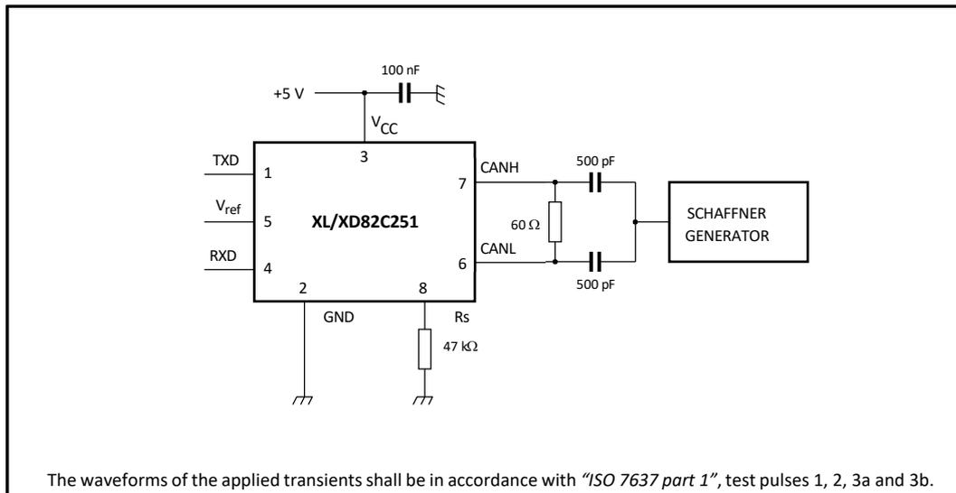
**Figure 6-6. Test circuit for transients**
