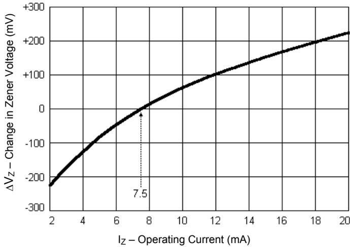
This curve in Figure 2 illustrates the change of diode voltage arising from the effect of impedance. It is in effect, an exploded view of the zener operating region of the I-V characteristic.
