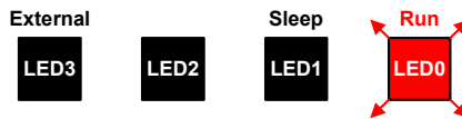
With PWM signals present on LI and HI, the Run LED is blinking
