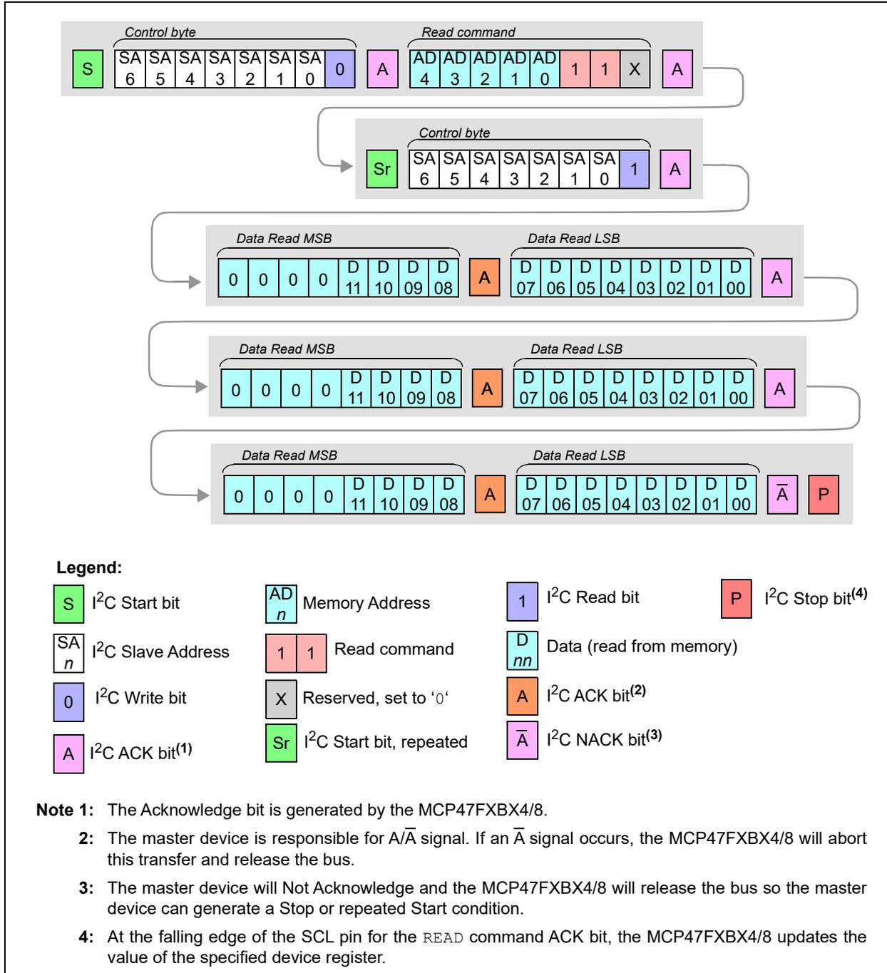
**FIGURE 7-7:** Continuous READ Command of Specified Address.
