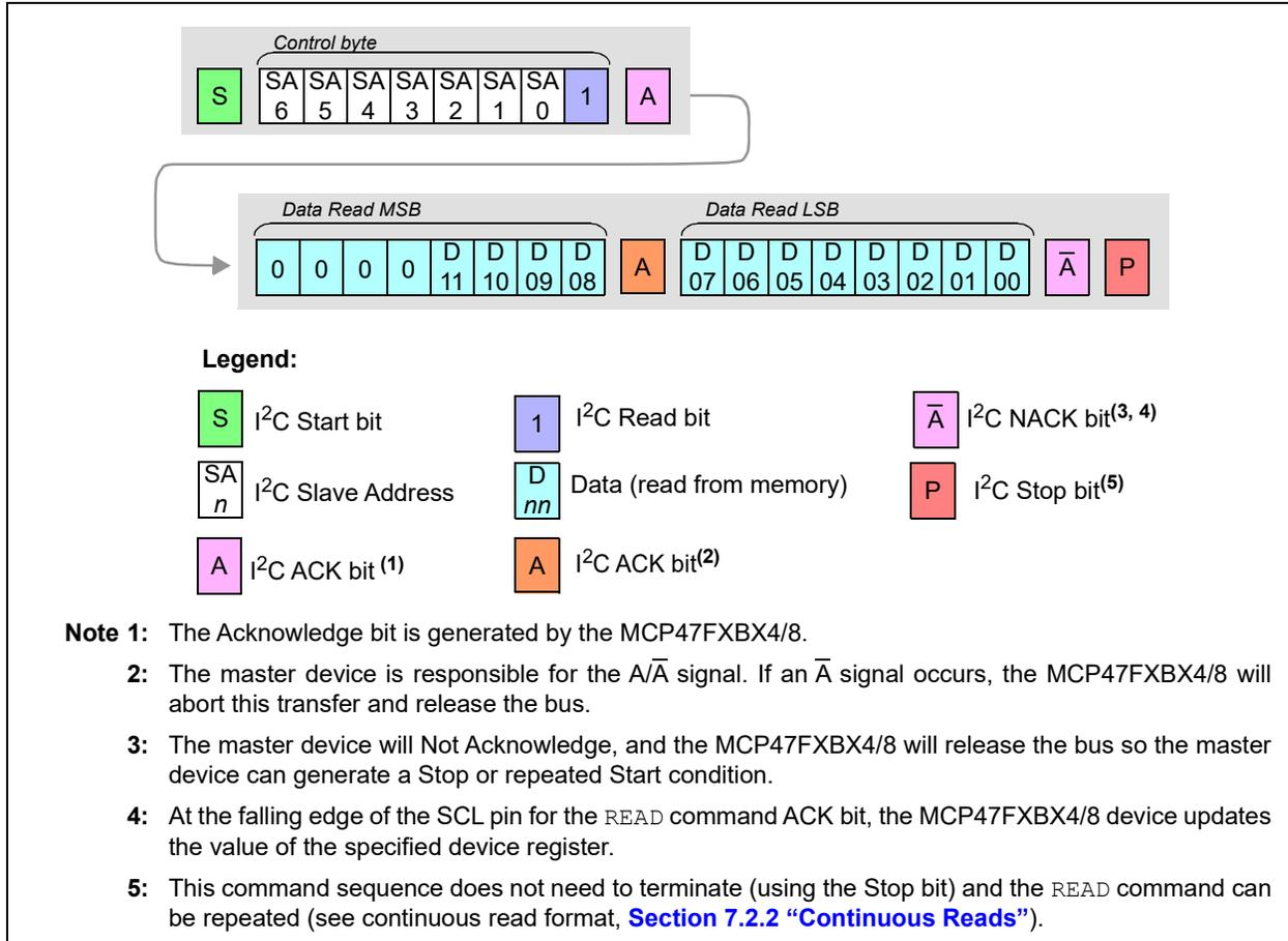
**FIGURE 7-5:** READ Command – Last Memory Address Accessed.
