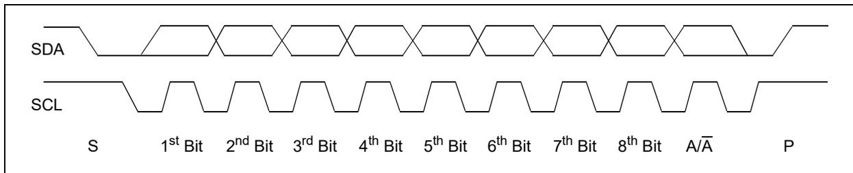
**FIGURE B-7: TYPICAL 8-BIT I<sup>2</sup>C WAVEFORM FORMAT.**
