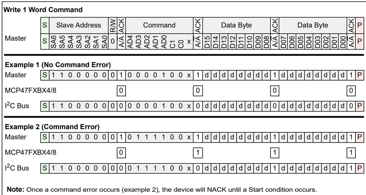
**FIGURE 7-2:** I<sup>2</sup>C ACK/NACK Behavior (Write Command Example).
