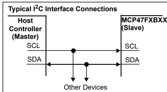
**FIGURE 6-1:** Typical I<sup>2</sup>C Interface.
