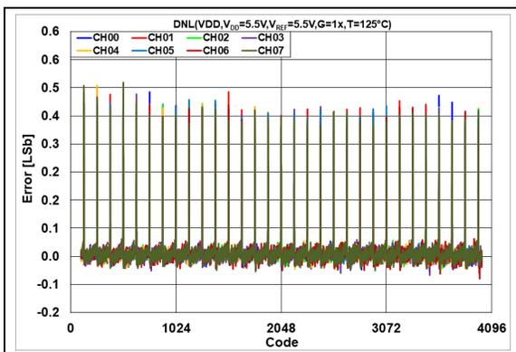
**FIGURE 2-25:** DNL Error vs. DAC Code,
