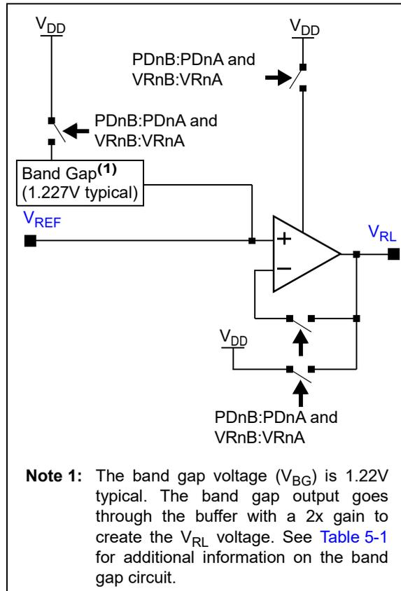
**FIGURE 5-4:** Reference Voltage Selection Implementation Block Diagram.
