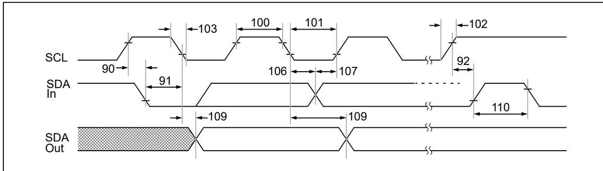
**FIGURE 1-7:** I<sup>2</sup>C Bus Timing Waveforms.
