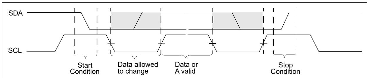
**FIGURE B-8: I<sup>2</sup>C DATA STATES AND BIT SEQUENCE.**
