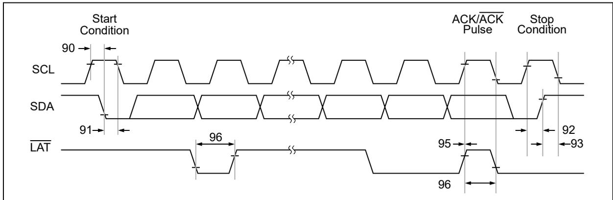
**FIGURE 1-5:** I<sup>2</sup>C Bus Start/Stop Bits and LAT Timing Waveforms.
