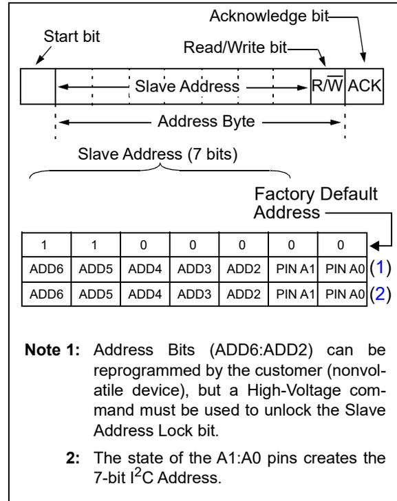
**FIGURE 6-2:** Slave Address Bits in the I<sup>2</sup>C Control Byte.
