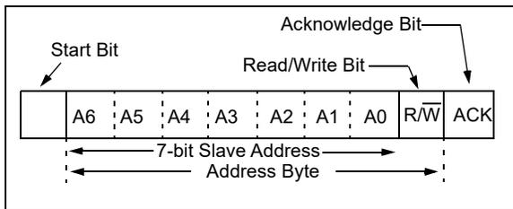
**FIGURE B-9: I<sup>2</sup>C SLAVE ADDRESS CONTROL BYTE.**
