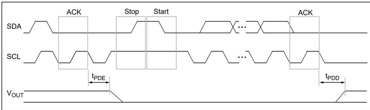
**FIGURE 1-4:** I<sup>2</sup>C Power-Down Command Waveforms.
