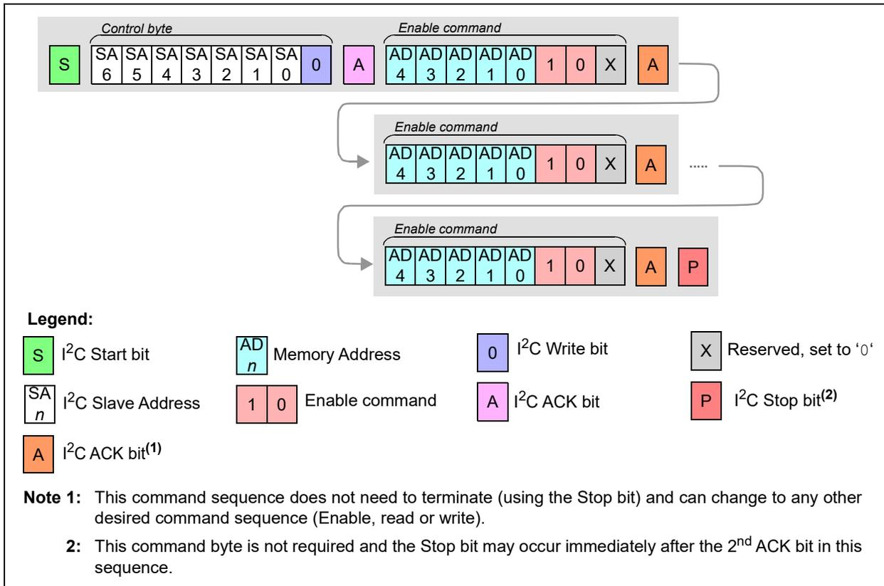
**FIGURE 7-11:** I<sup>2</sup>C Enable Command Sequence.
