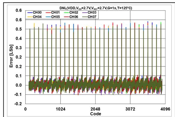
**FIGURE 2-28:** DNL Error vs. DAC Code,
