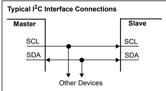
FIGURE B-1: TYPICAL I<sup>2</sup>C INTERFACE.
