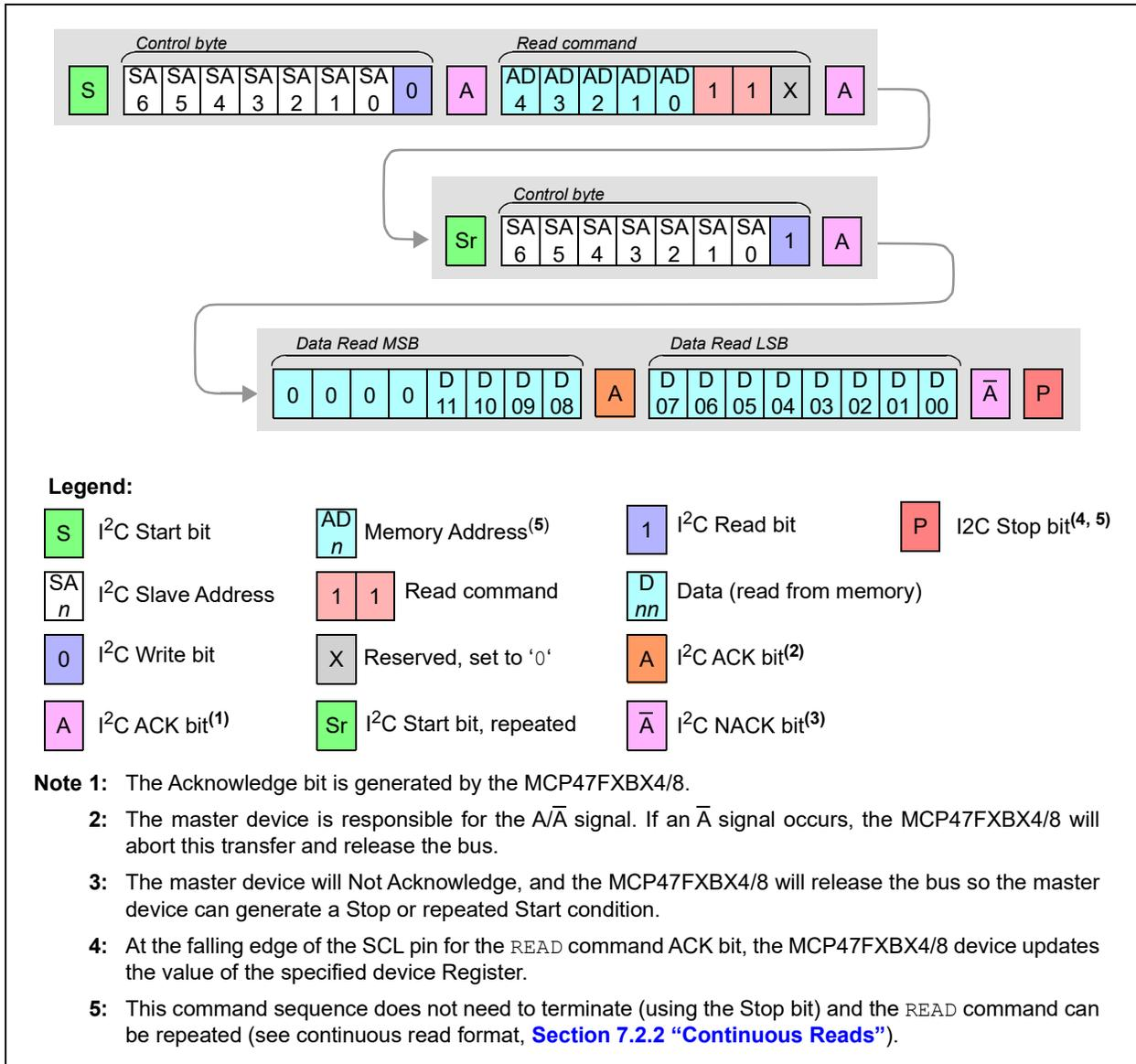
**FIGURE 7-4:** READ Command – Single Memory Address.
