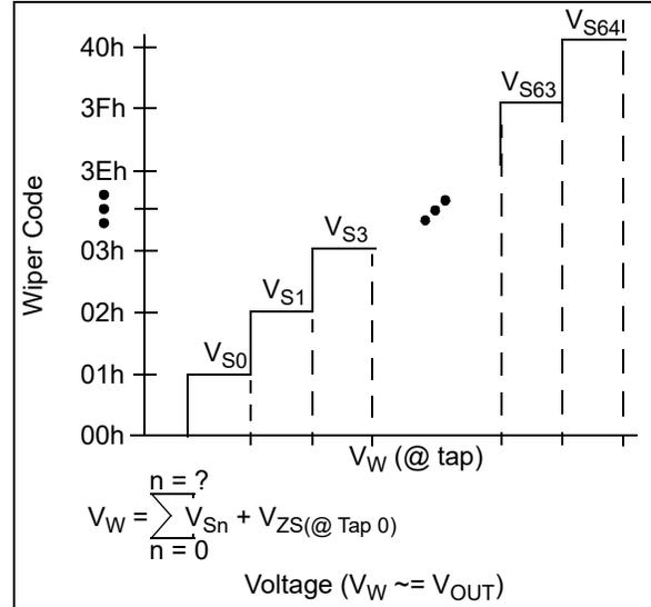
FIGURE C-1:  $V_W (V_{OUT})$ .
