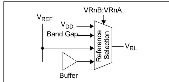
**FIGURE 5-3:** Resistor Ladder Reference Voltage Selection Block Diagram.
