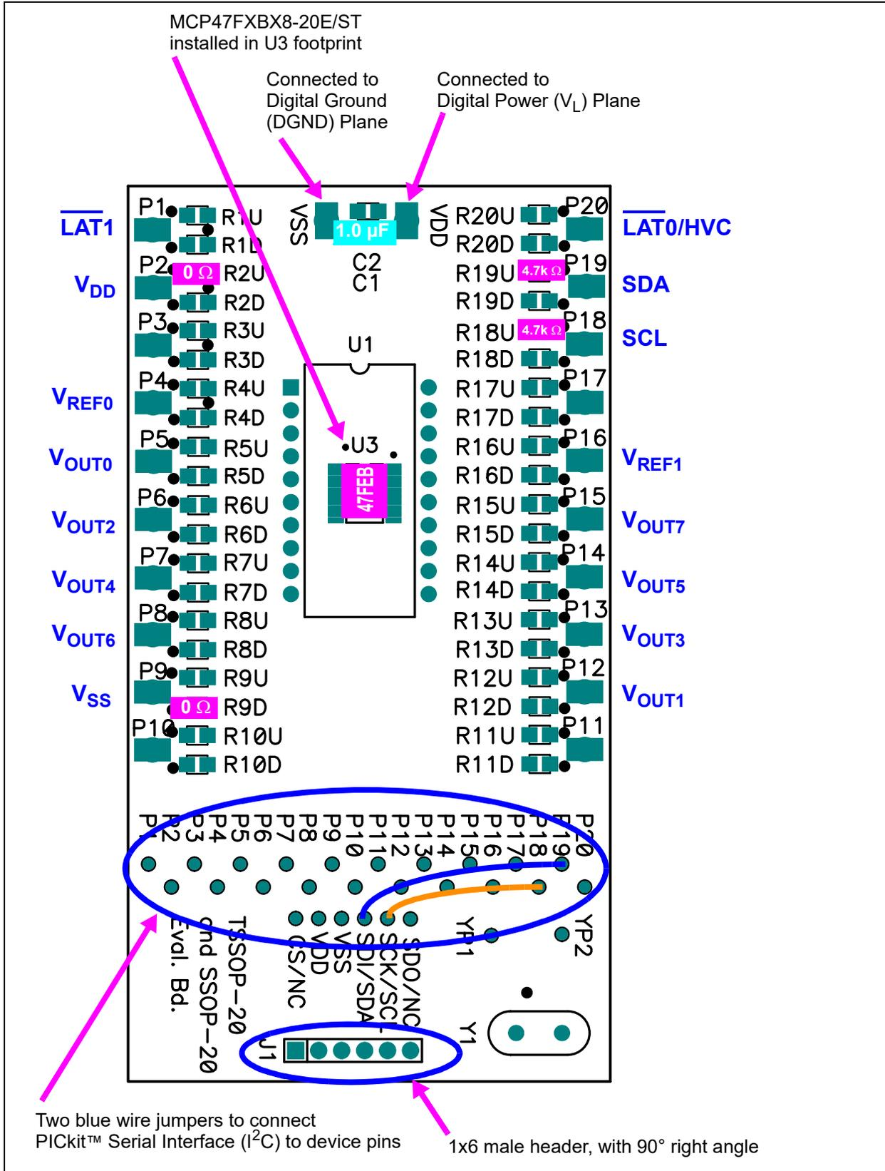
FIGURE 9-1: MCP47FBX4/8 Evaluation Board Circuit Using TSSOP20EV.
