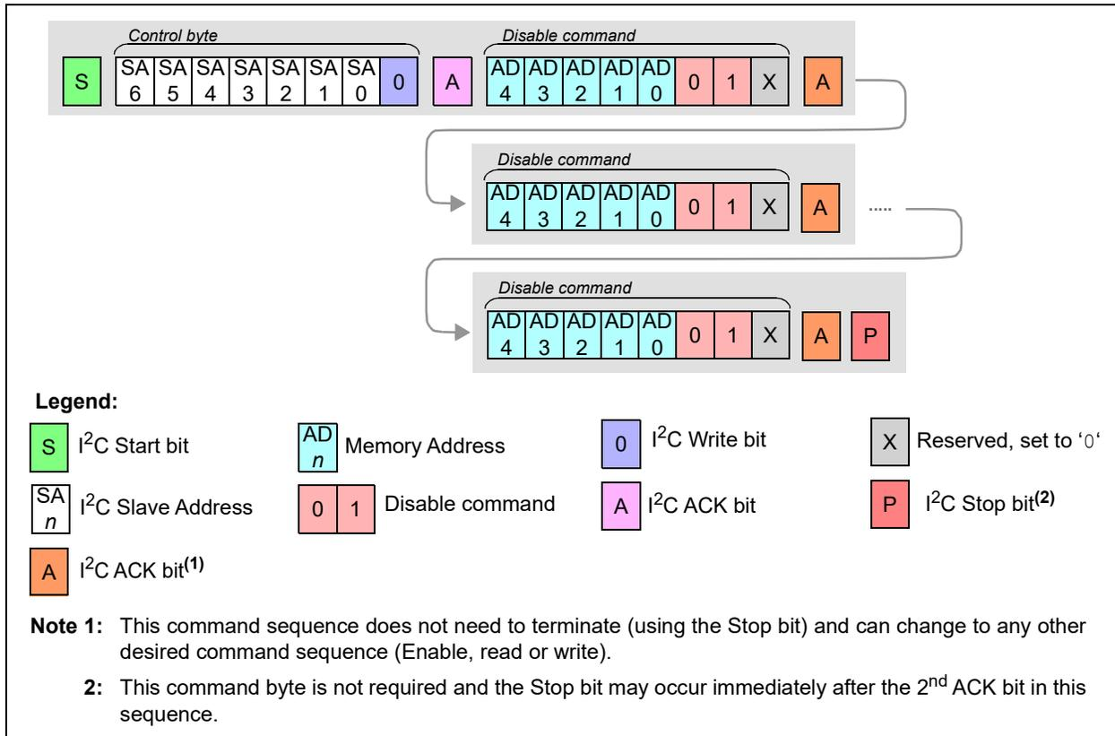
**FIGURE 7-12:** I<sup>2</sup>C Disable Command Sequence.
