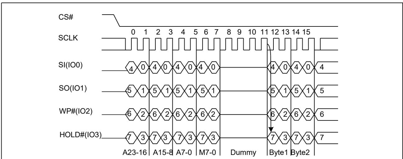
**Quad I/O Fast Read with “8/16/32/64-Byte Wrap Around” in Standard SPI mode**
