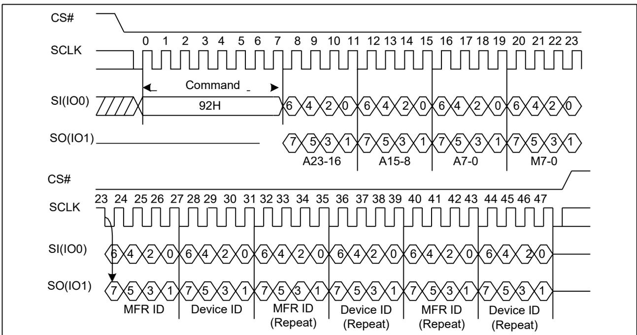
**7.24 Read Manufacture ID/ Device ID Quad I/O (94H)**
