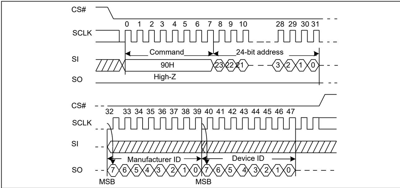
**7.23 Read Manufacture ID/ Device ID Dual I/O (92H)**
