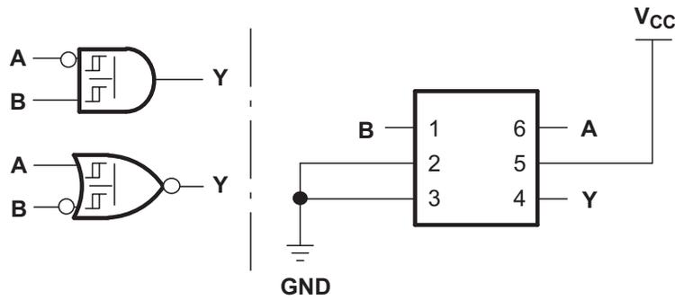
Figure 6. 2-Input AND Gate With One Inverted Input
