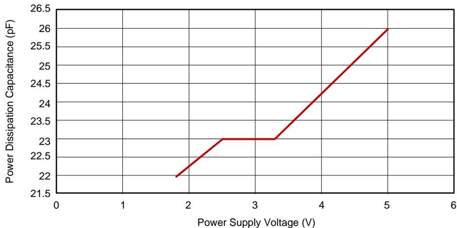
Figure 1. Power Dissipation Capacitance vs Power Supply Voltage
