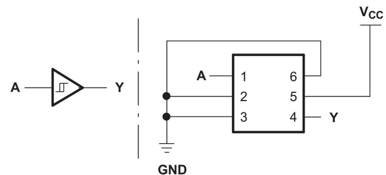
Figure 9. Noninverted Buffer
