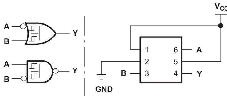
**Figure 5. 2-Input OR Gate With One Inverted Input
