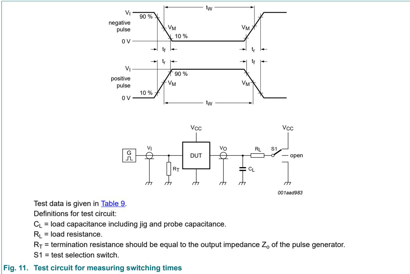
Fig. 11. Test circuit for measuring switching times
