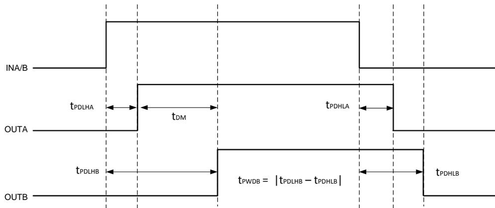
图 27. Delay Matching and Pulse Width Distortion
