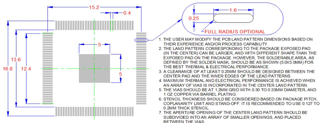
**PCB LAND PATTERN AND APPLICATION NOTES****Figure 6 LAN9311/LAN9311i 128-XVTQFP Recommended PCB Land Pattern**
