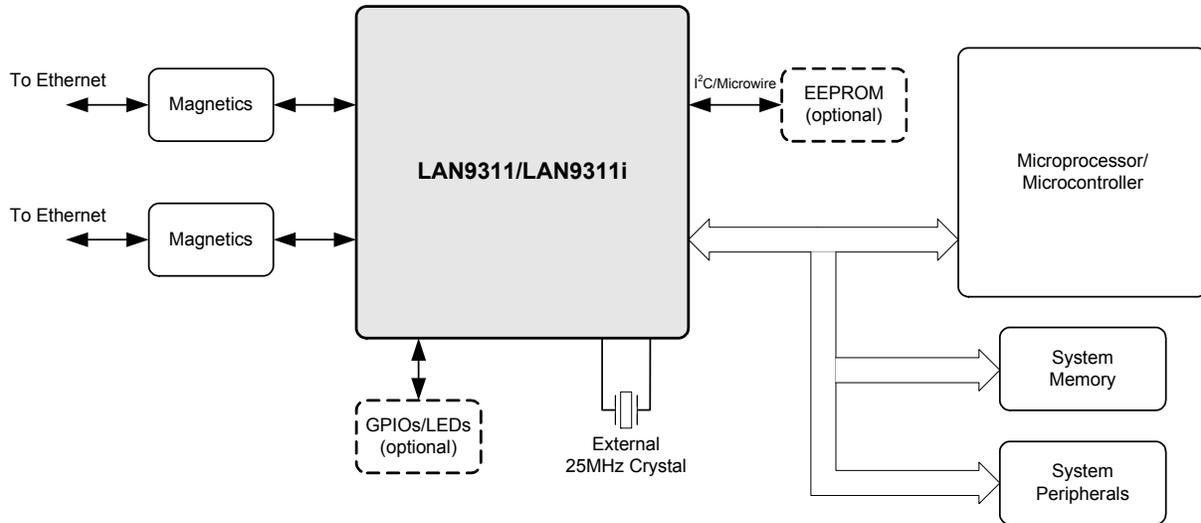
Figure 1 System Level Block Diagram Utilizing the LAN9311/LAN9311i
