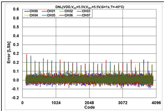
**FIGURE 2-23:** DNL Error vs. DAC Code,
