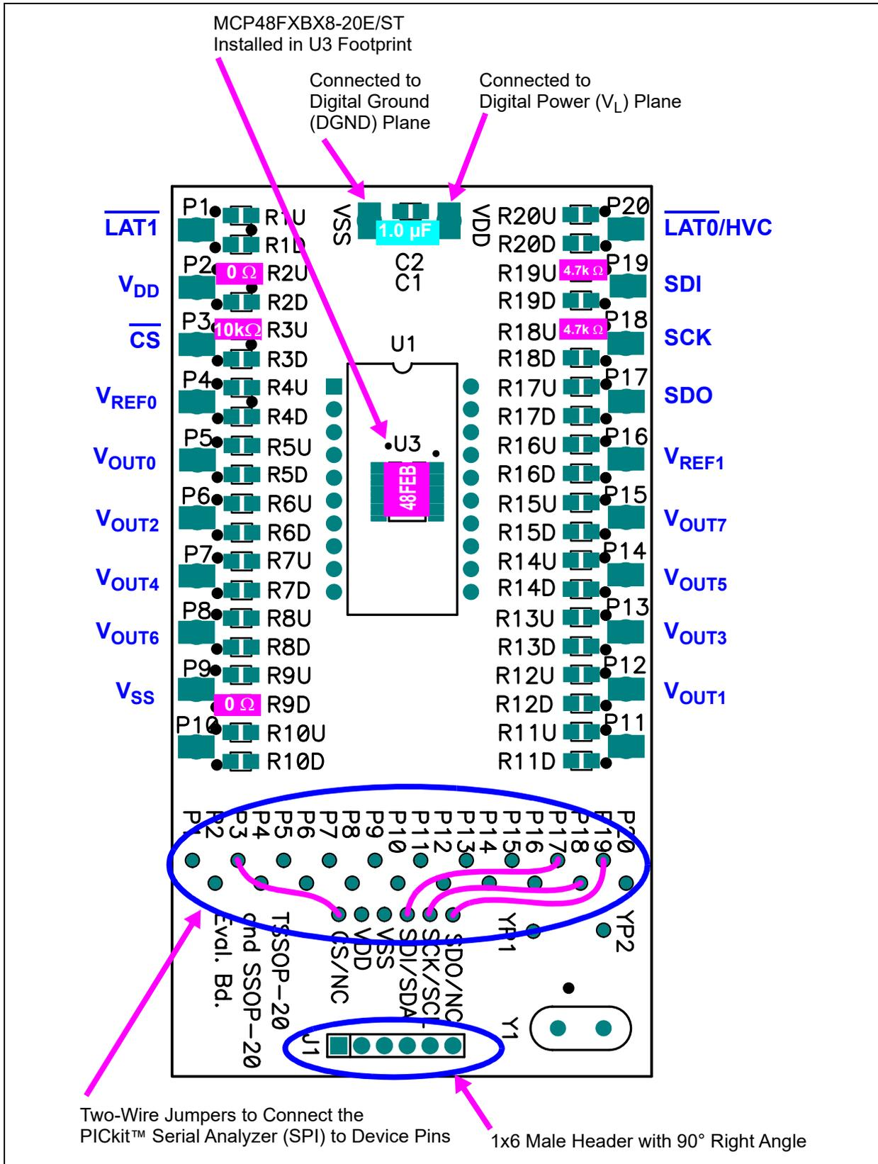
FIGURE 9-1: MCP48FBX4/8 Evaluation Board Circuit Using TSSOP20EV.
