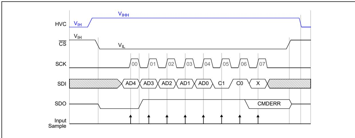
**FIGURE 7-16:** 8-Bit Disable Command ( $C1:C0 = 01$ ) – SPI Waveforms (Mode 0,0).
