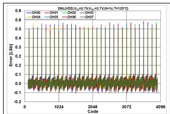
**FIGURE 2-28:** DNL Error vs. DAC Code,
