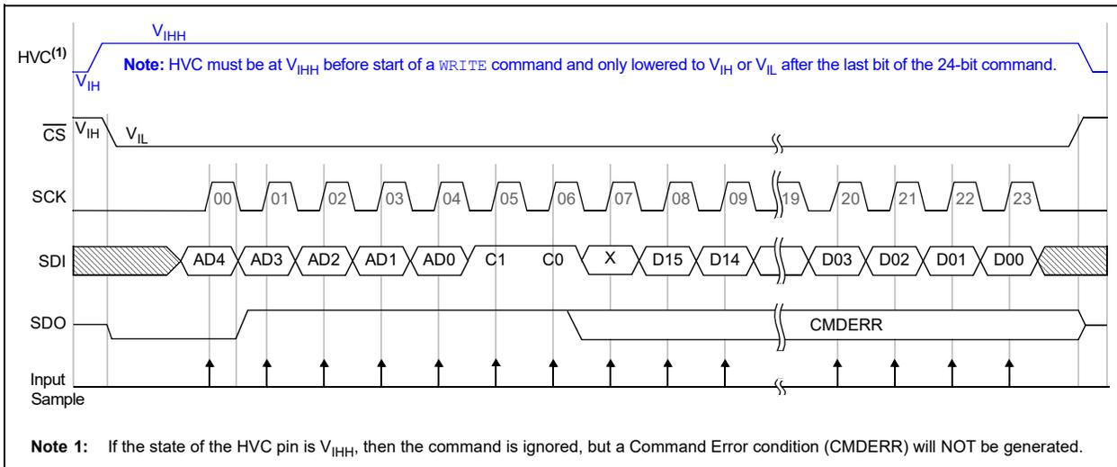
**FIGURE 7-10:** 24-Bit READ Command ( $C1:C0 = 11$ ) – SPI Waveforms (Mode 0,0).
