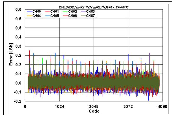
**FIGURE 2-26:** DNL Error vs. DAC Code,
