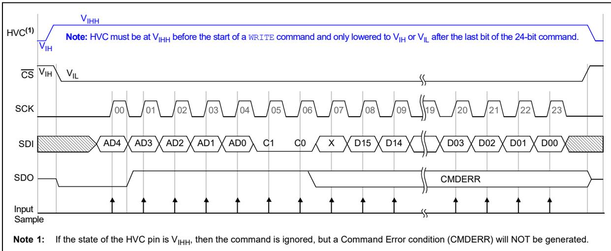
**FIGURE 7-5:** 24-Bit `WRITE` Command ( $C1:C0 = 00$ ) – SPI Waveform (Mode 0,0).
