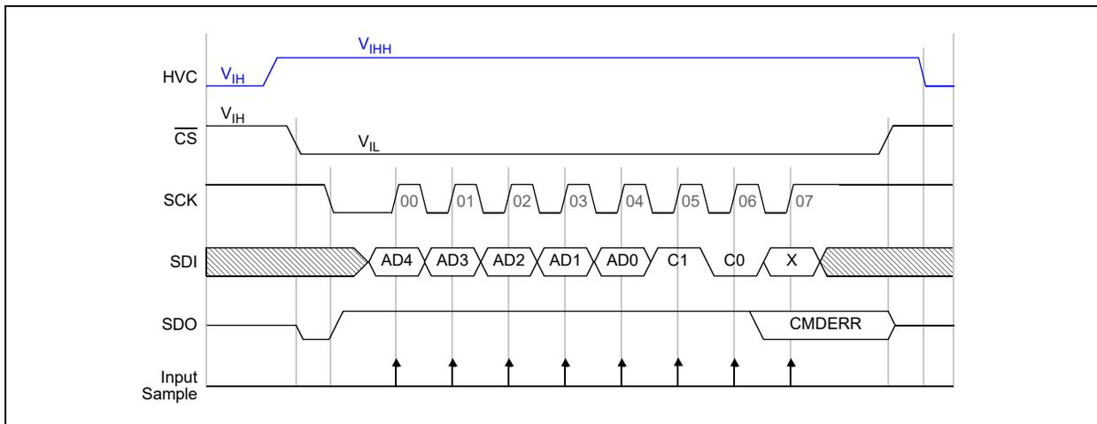
FIGURE 7-12: 8-Bit Enable Command (C1:C0 = 10) – SPI Waveforms (Mode 1,1).
