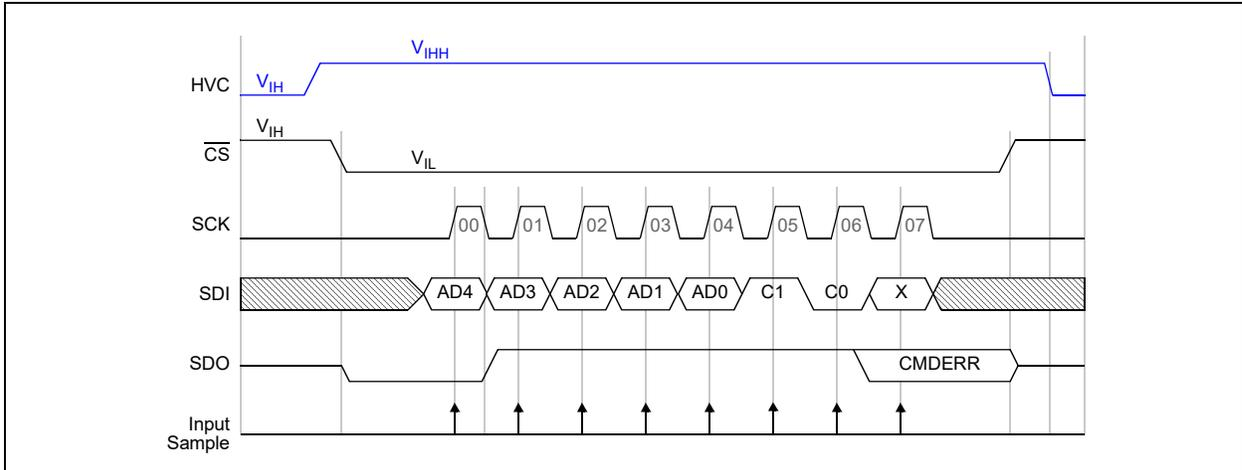
**FIGURE 7-13:** 8-Bit Enable Command (C1:C0 = 10) – SPI Waveforms (Mode 0,0).
