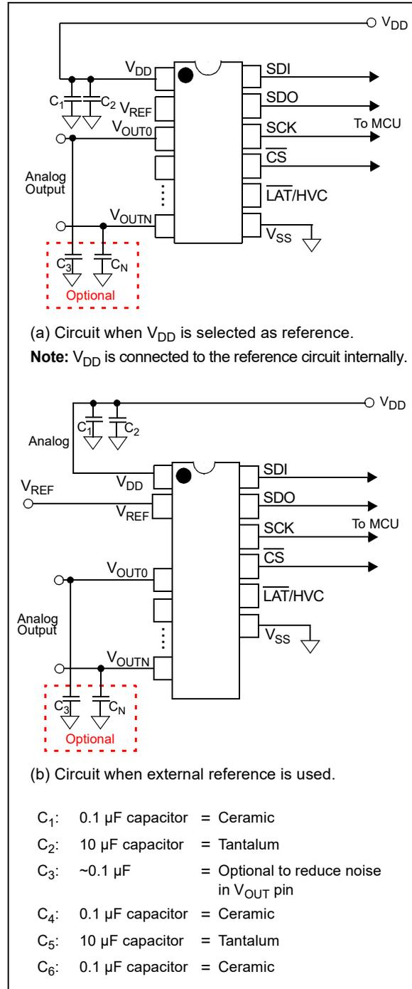
**FIGURE 8-1:** Example Circuit.
