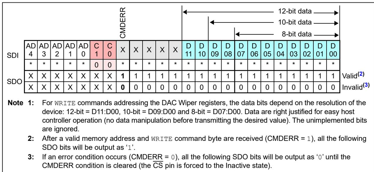
**FIGURE 7-3:** Write Single Memory Location Command – SDI and SDO States.<sup>(1)</sup>
