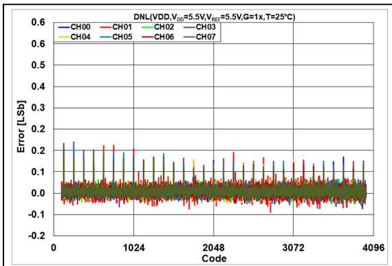
**FIGURE 2-24:** DNL Error vs. DAC Code,
