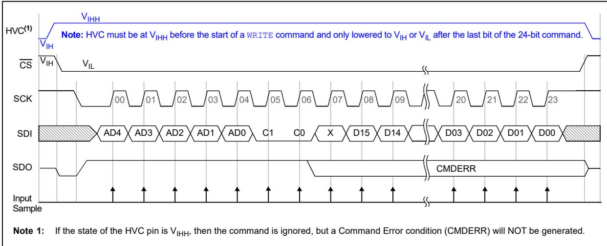
**FIGURE 7-4:** 24-Bit `WRITE` Command ( $C1:C0 = 00$ ) – SPI Waveform (Mode 1,1).
