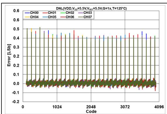
**FIGURE 2-25:** DNL Error vs. DAC Code,
