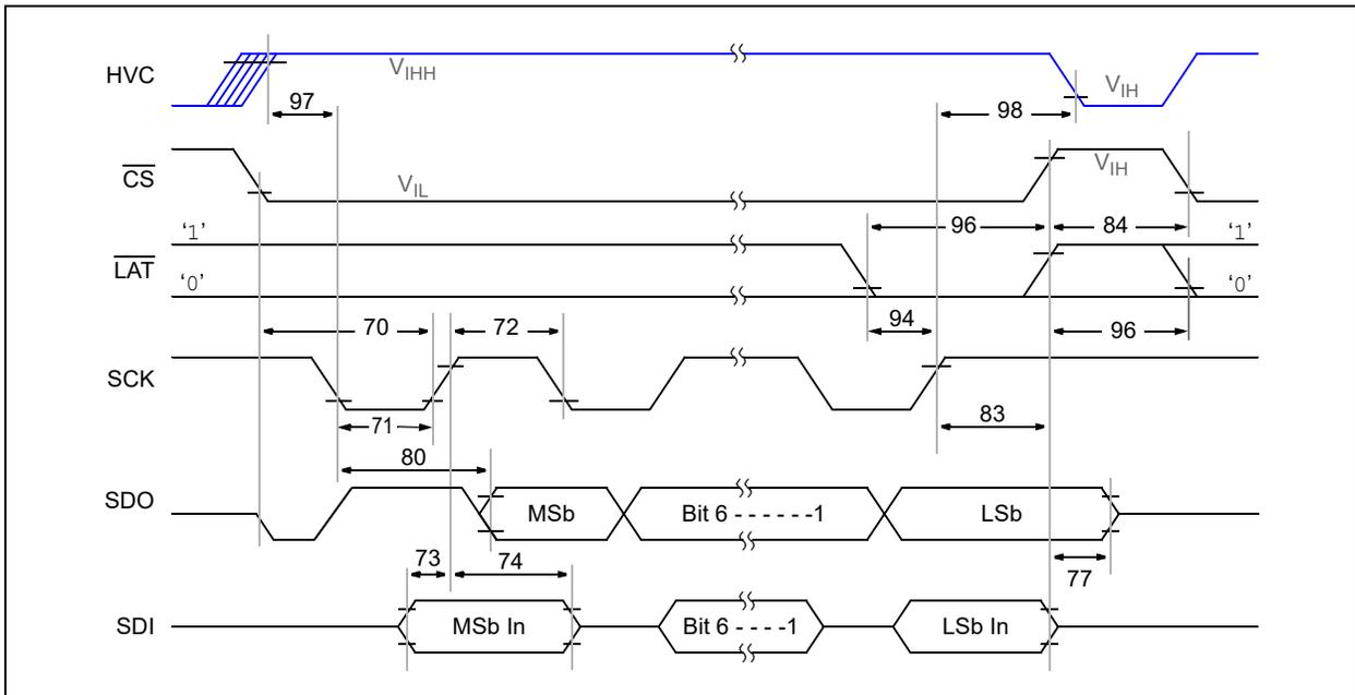
**FIGURE 1-5:** SPI Timing Waveforms – Mode 1,1.
