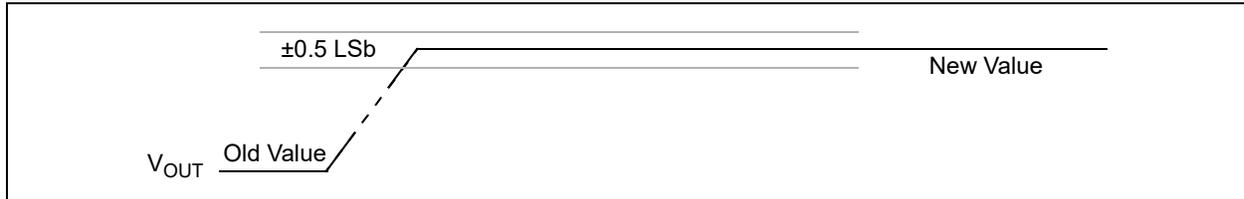
**FIGURE 1-1:**  $V_{OUT}$  Settling Time Waveforms.
