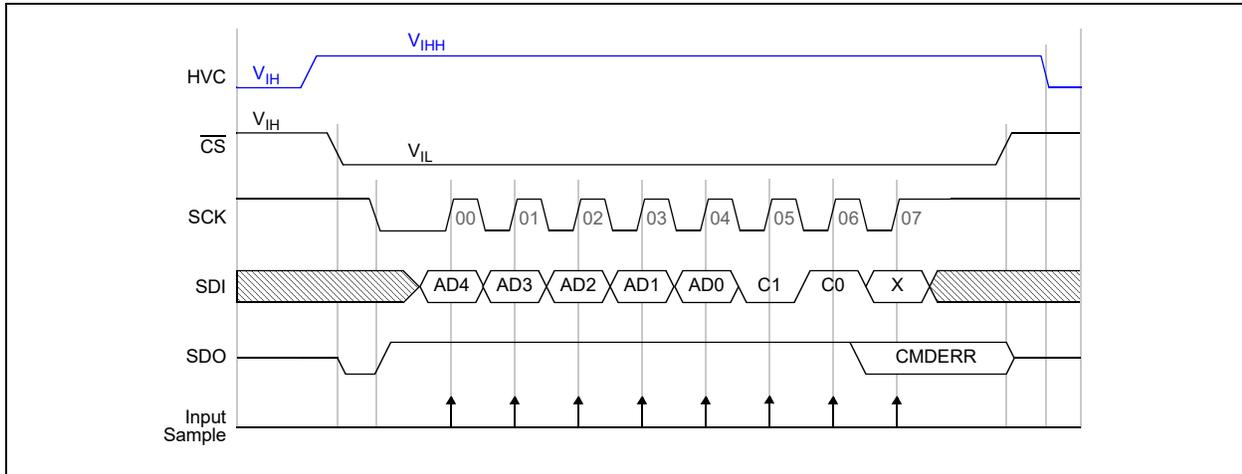
**FIGURE 7-15:** 8-Bit Disable Command ( $C1:C0 = 01$ ) – SPI Waveforms (Mode 1,1).
