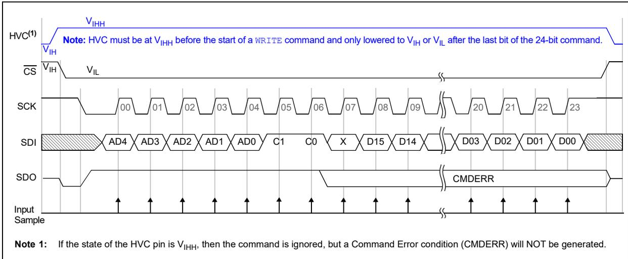
**FIGURE 7-9:** 24-Bit READ Command ( $C1:C0 = 11$ ) – SPI Waveforms (Mode 1,1).
