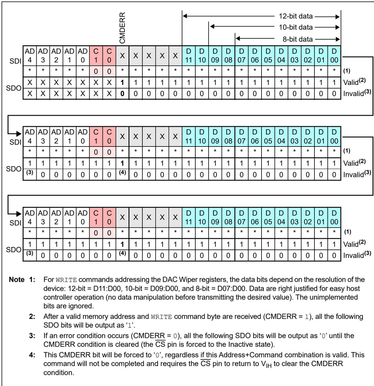
**FIGURE 7-6:** Continuous WRITE Commands (Volatile Memory Only).
