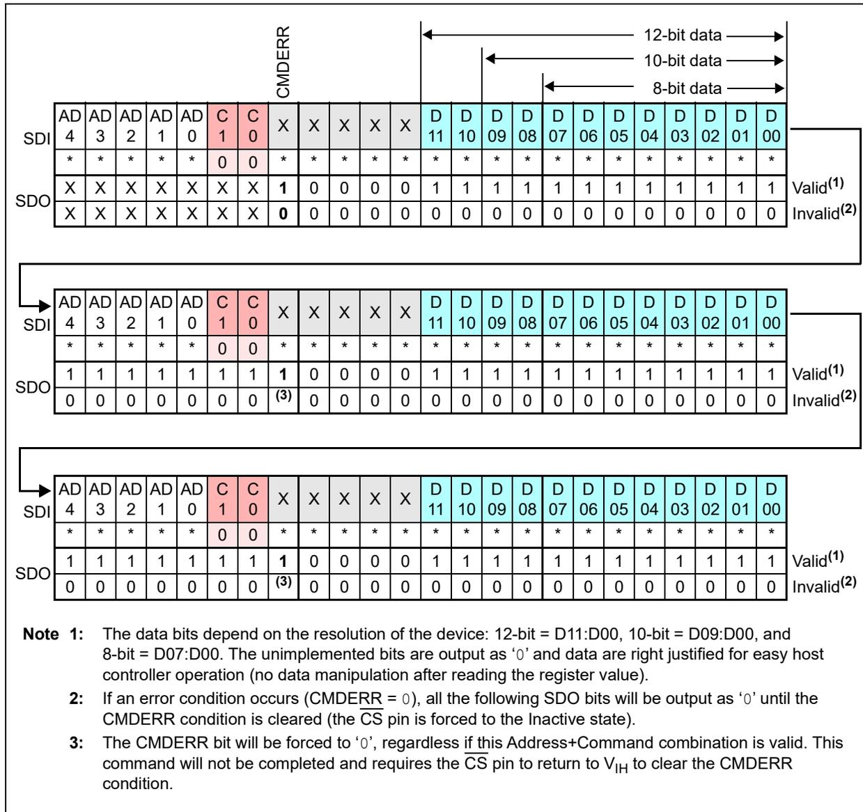
FIGURE 7-8: READ Command – Continuous Read Sequence.
