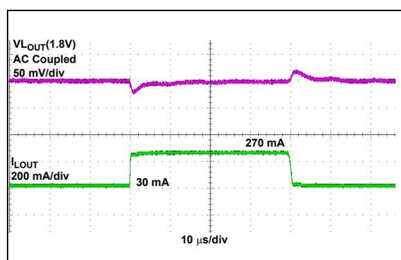
**FIGURE 2-18:** LDO Load Transient Response.
