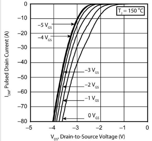
Figure 10 •  $I_D$  vs.  $V_{DS}$  3<sup>rd</sup> Quadrant Conduction
