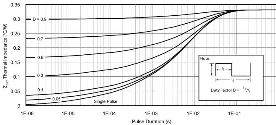
Figure 20 • Maximum Transient Thermal Impedance
