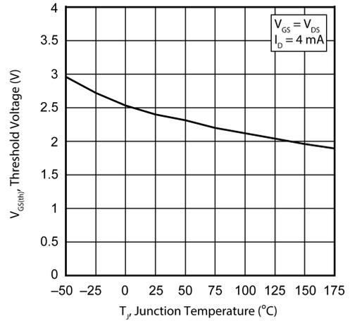
Figure 18 • Threshold Voltage vs. Junction Temp.
