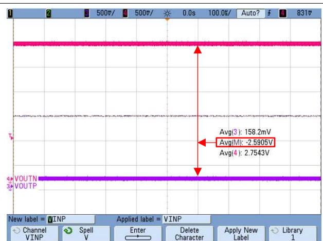
Figure 48. Typical Failsafe Output of the AMC1301
