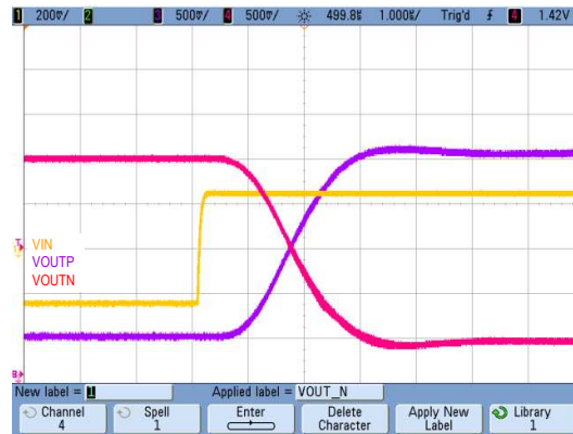
Figure 50. Step Response of the AMC1301
