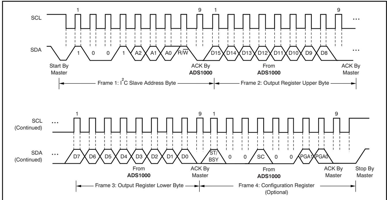
Figure 7. Timing Diagram for Reading from the ADS1000
