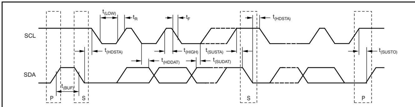
Figure 6. I<sup>2</sup>C Timing Diagram
