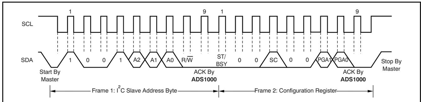
Figure 8. Timing Diagram for Writing to the ADS1000
