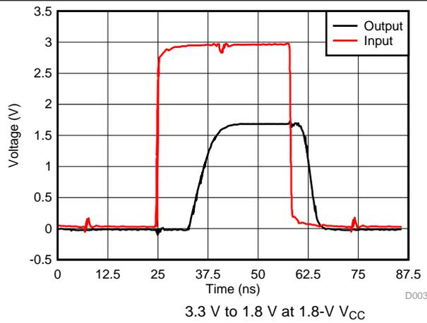
**Figure 4. Switching Characteristics at 15 MHz
