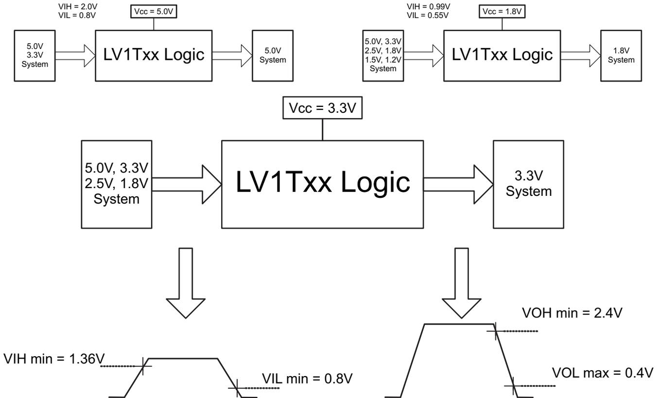
Figure 1. Switching Thresholds For 1.8-V to 3.3-V Translation
