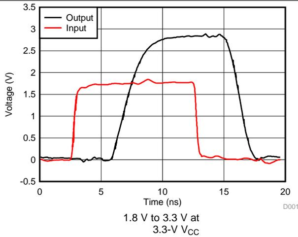
**Figure 2. Switching Characteristics at 50 MHz
