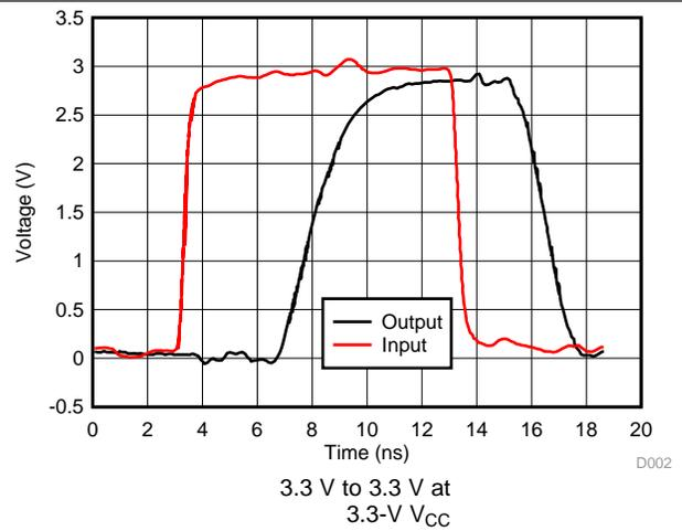
**Figure 3. Switching Characteristics at 50 MHz
