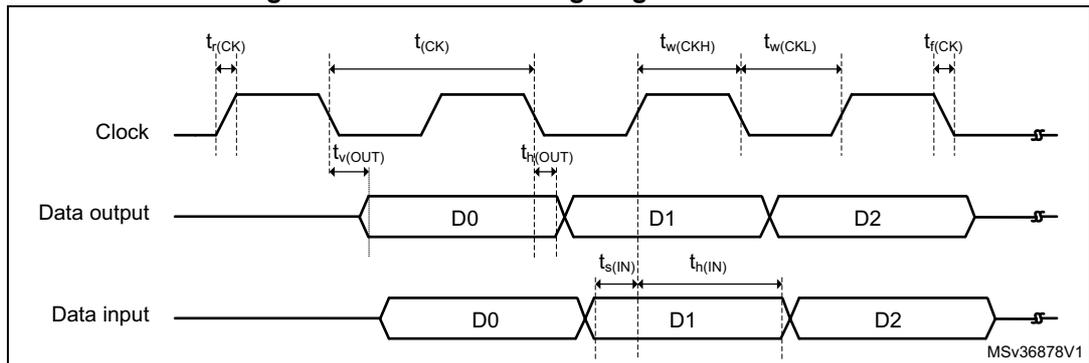
Figure 37. Quad-SPI timing diagram - DDR mode
