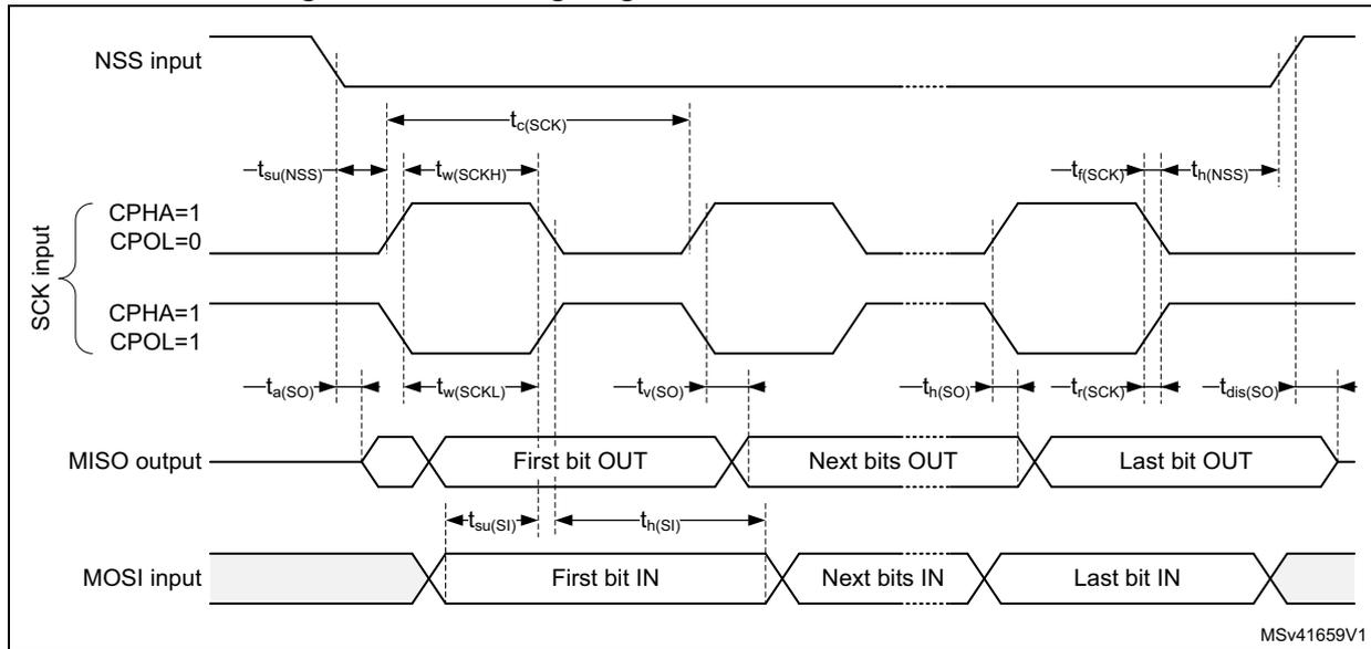
1. Measurement points are done at 0.5V<sub>DD</sub> and with external C<sub>L</sub> = 30 pF.
