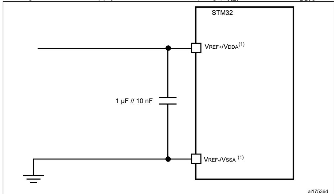
1.  $V_{REF+}$  input is available on all package whereas the  $V_{REF-}$  s available only on UFBGA176+25 and TFBGA240+25. When  $V_{REF-}$  is not available, it is internally connected to  $V_{DDA}$  and  $V_{SSA}$ .
