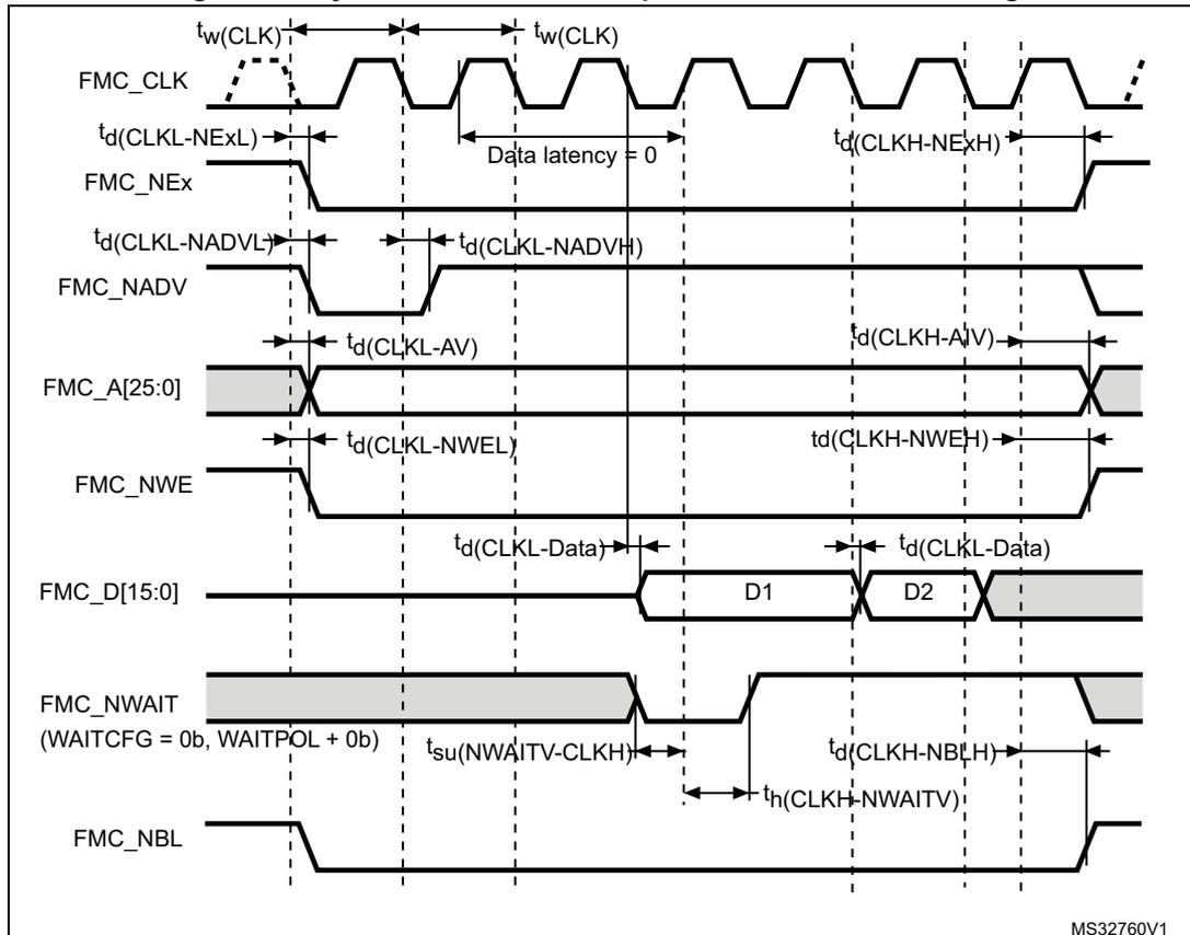
Table 74. Synchronous non-multiplexed PSRAM write timings<sup>(1)</sup>
