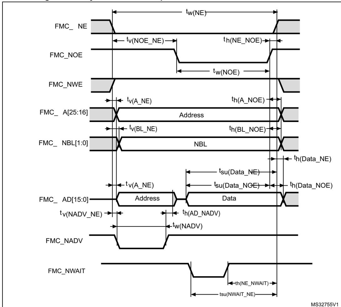
**Table 67. Asynchronous multiplexed PSRAM/NOR read timings<sup>(1)</sup>**
