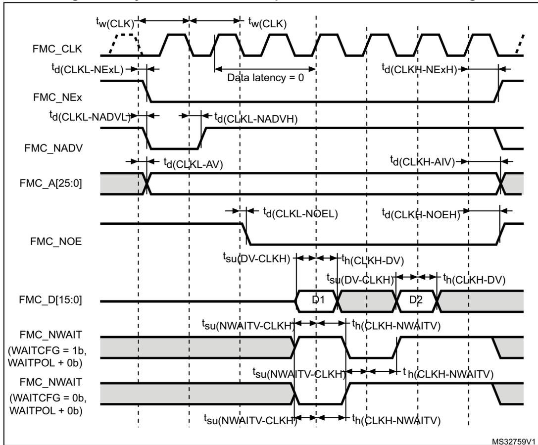
Table 73. Synchronous non-multiplexed NOR/PSRAM read timings<sup>(1)</sup>
